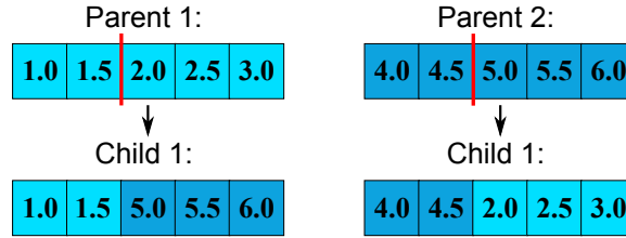
Figure 4.2 Illustration of the single point crossover with the 3rd variable chosen as the crossover point.
